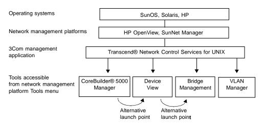
Figure 3-1 UNIX Tools for Configuring ATM Backbone SwitchModules
